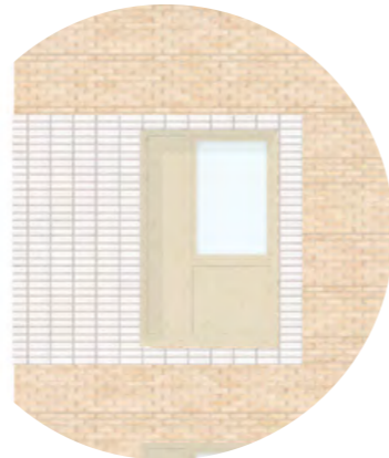
"Corner" Windows Brick Surround
