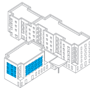
4 Natural ventilation maximising dual aspect Window sizes to vary depending on aspect
