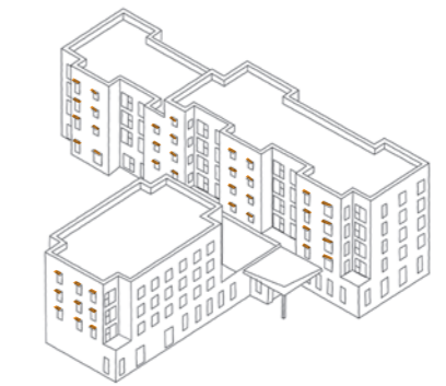
6 Solar shading above balconies and south and west facing windows
